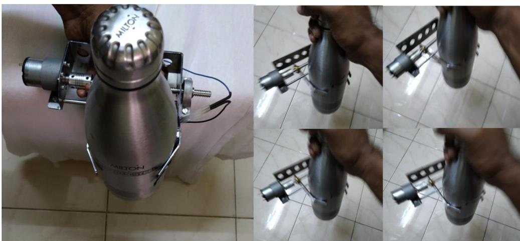
Figure 14. L.S.Gripper performance verification with Milton bottle
