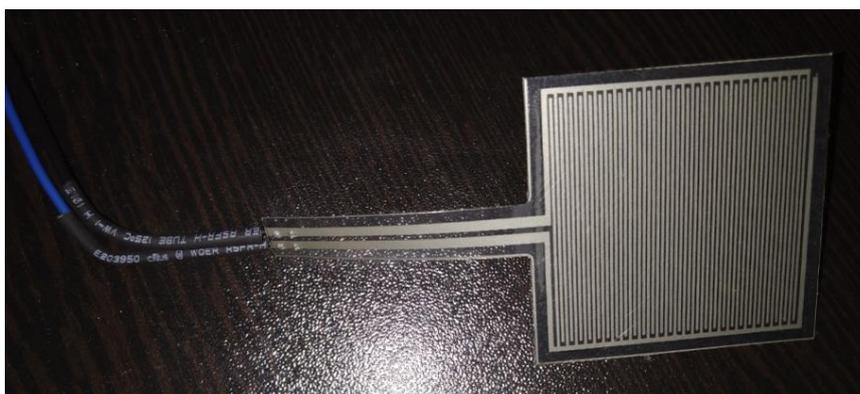
Figure 6. Force sensitive resistor, 40x40 mm area
